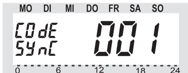
Now you need to synchronise the (first) valve operating mechanism ('001' on the display) to the new security code. Proceed as follows to carry out this synchronisation:
